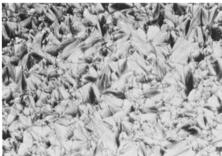
Figure 3. A typical focal-conic texture of the smectic A phase of monomer 9b .
