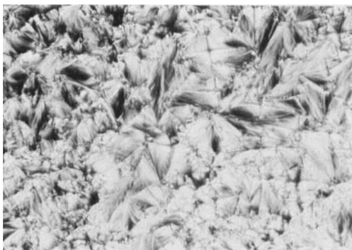
Figure 4. The broken focal-conic fan texture of the smectic C^* phase of monomer 9b .
